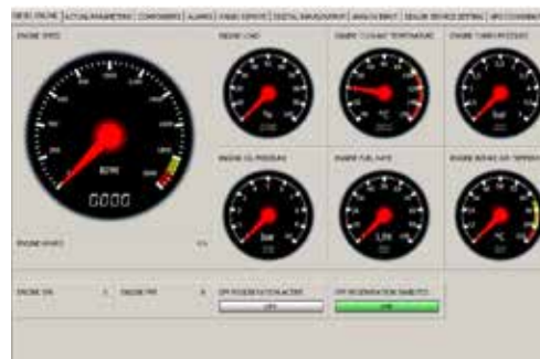
Real Time Access of Remote Control Application, here showing the Diesel Engine page
