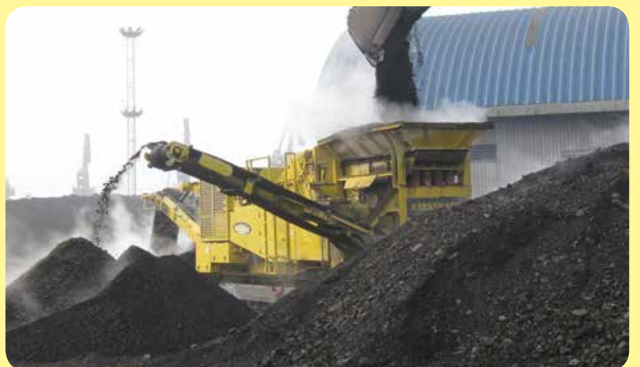
Destroyer 1112 impact crusher, crushing coal in China up to 400t/h
