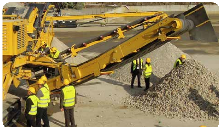
Destroyer 1113 swiveling return conveyor to stockpile conveyor
