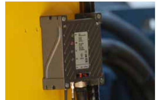
Remote Control Application with GPS using GSM/UMTS modem and combined GSM/GPS antenna
