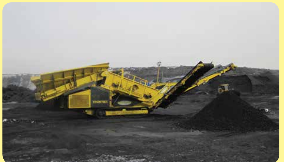
Frontier screening coal in China up to 500 ton/hour
