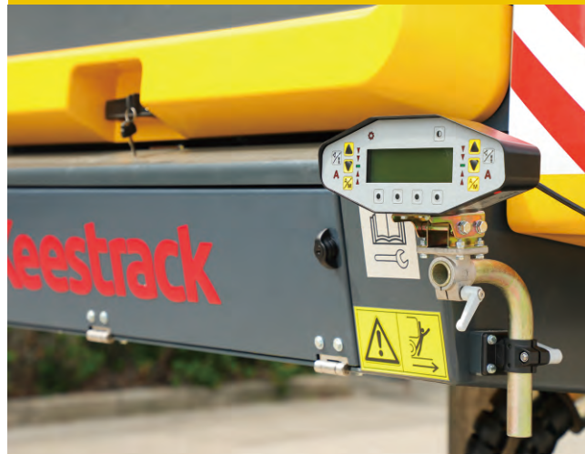
GROUND LEVEL CONTROL
