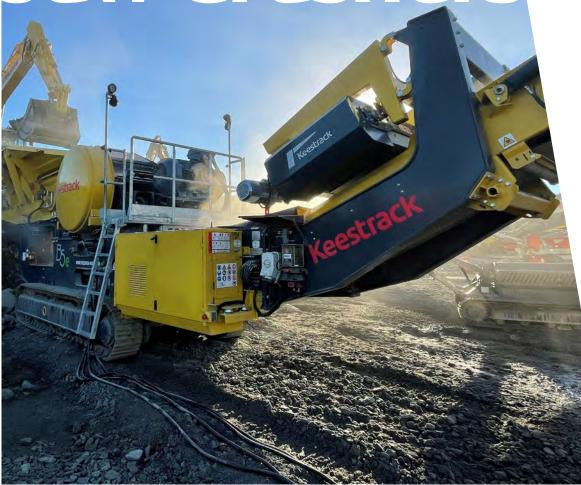
**Jaw crushers** are often used as primary crushers in recycling, quarrying, and mining applications.
