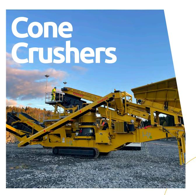
**Cone crushers** are used in secondary, tertiary, or quaternary crushing applications in quarrying & mining and aggregate production. All Keestrack cone crushers are equipped with a metal detector to protect the cone.
